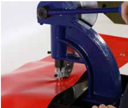
Riveting and piercing in one single step
